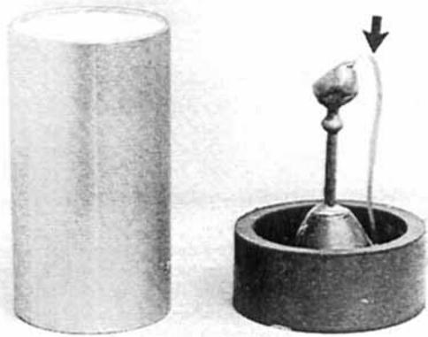
Fig. 1. Investing ring with fiberglass lining and wax model with air vent (arrow) mounted for investing.
