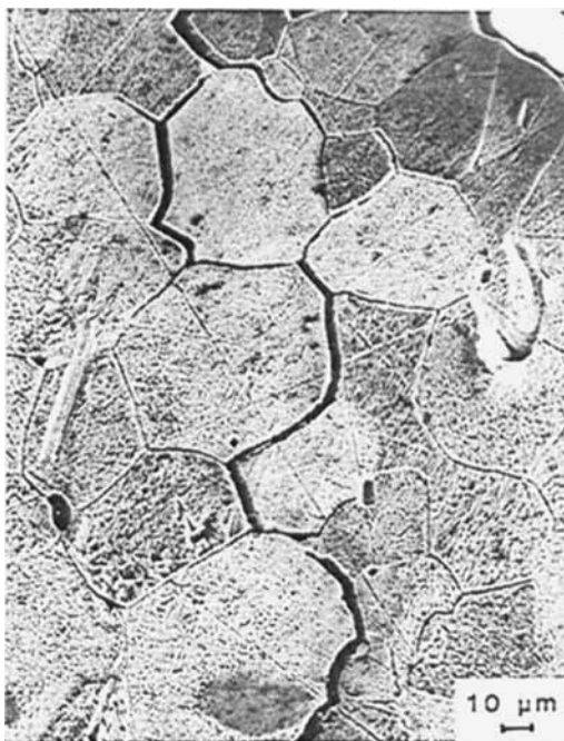
Fig. 4. A small branch of the crack shown in Fig. 3.
