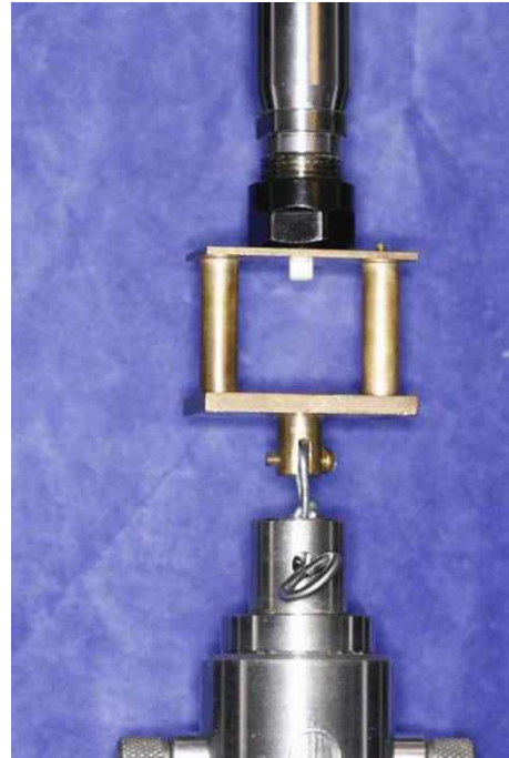
Figure 4. The ATS set-up. The specimen was placed in a jig, which fixed the resin composite core and the non-embedded part of the post.
