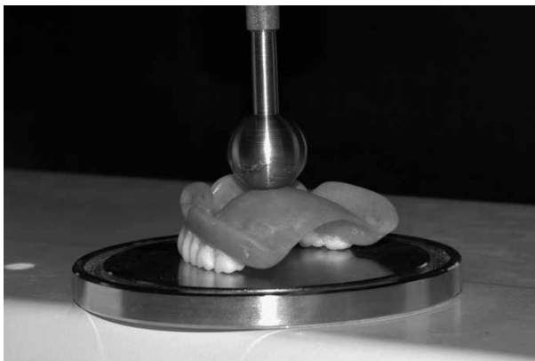
Figure 3. Fracture strength test using compression load assembly.
