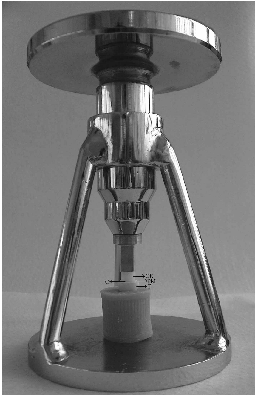
Figure 1. Experimental set-up with special loading device (CR: ceramic, C: cement, PM: polyethylene mold, T: tooth).
