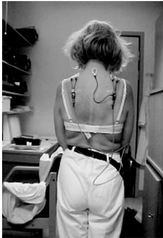
Figure 1. The MyoGuard system. A portable EMG equipment for collection and on-line processing of myoelectric signals. The figure shows electrode placement over the left and right trapezius muscles and the datalogger unit on the right side of the hip.
