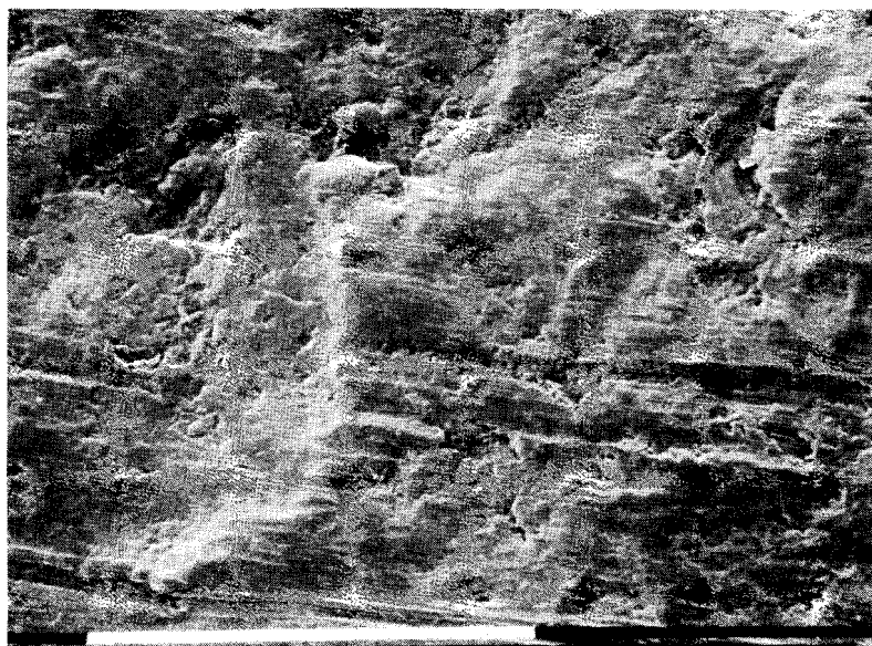
Fig. 6. Resin denture tooth antagonizing heat-cured resin for 2 months (white line = 0.1 mm).
