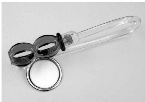
Fig. 1. The specially made plastic clip with the 18-mm paper disk and aluminum cap.
