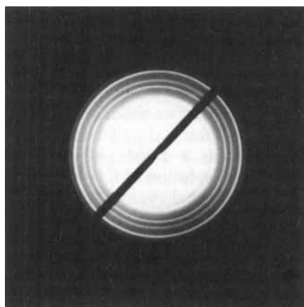
Fig. 7. Electron diffraction pattern of \text{CaF}_2(\text{P}) -2. In this figure 1.0 cm represents 1.0 cm, and the d spacings can be calculated from eqn. (6).
