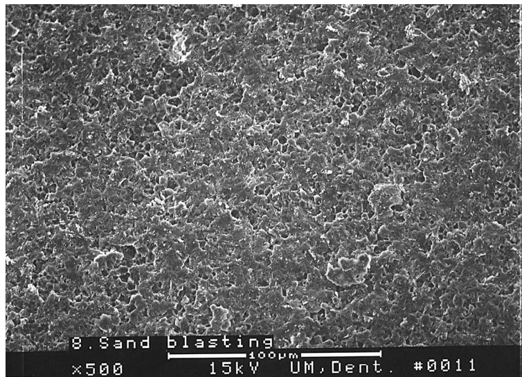
Fig. 3. Scanning electron microscope photograph of alumina oxide core material after sandblasting with 50- \mu m aluminum oxide.
