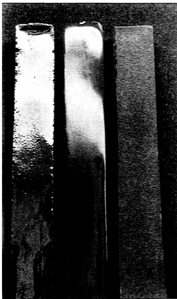
Fig. 2. Photograph of test specimens. From the left: light-curing resin-coated (group 3), rag-wheel-polished (group 2), and untreated (group 1) specimens.
