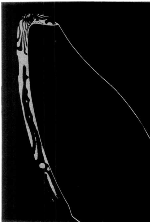
Fig. 7. Type-1 thinned facing, lamination H, inclination 30°.
