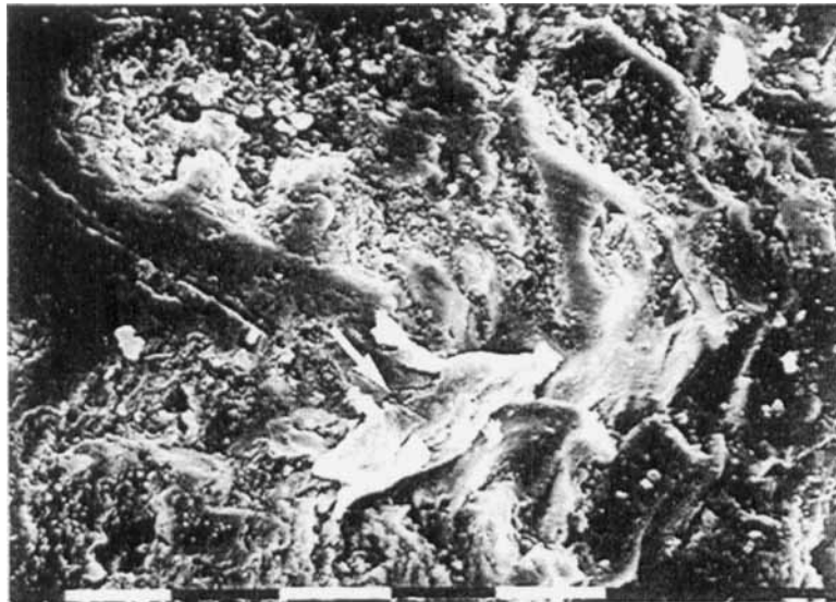
Fig. 9. Occlusal contact area of porcelain after 1 month's exposure to the oral environment, right-side segment. Horizontal bar corresponds to 10 \mu m.
