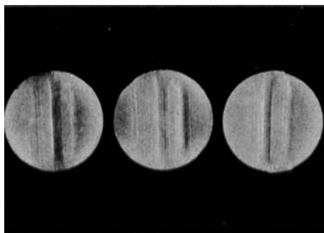
Fig. 2. Acrylic resin specimens abraded by tooth-brushing under conditions described in the text.
