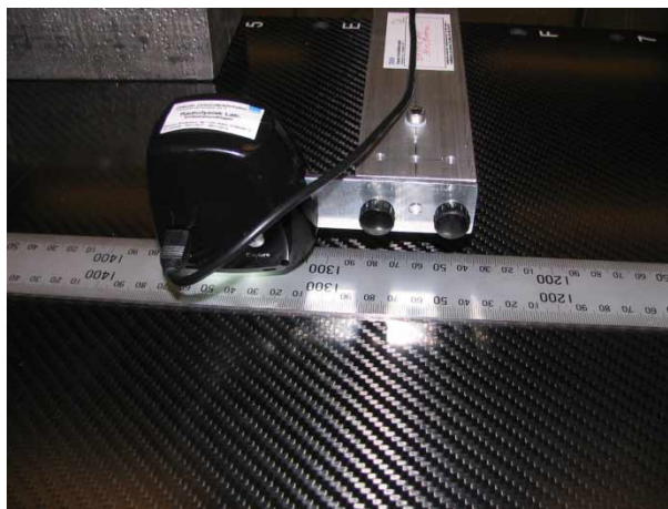
Figure 1. Experimental set-up for the longitudinal measurements on Ac4 with the 2000 mm ruler aligned on the table top. The black housing is the USB-microscope from Spectrum Technologies, Inc. The 8 cm aluminium arm was mounted via two thumbscrews at the end of a 25 \times 50 mm 2 massive aluminium bar of length 124 cm (weight 4.2 kg). A PTW MP3 water phantom was used as elevation stage for aluminium bar with the microscope mounted at the end.
