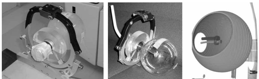
Figure 2. From left: gel filled phantom with the stereotactic frame in the treatment position on the accelerator. Phantom with LIC mounted. 3D reconstruction from the CT study of the phantom with the LIC.
