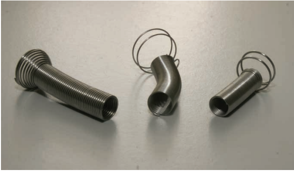
Figure 1. Three different stent designs have been investigated. To the left is the Memokath, which was developed for treatment of benign prostate hyperplasia. In the middle is the DS-I stent. To the right is the DS-II stent, which currently is being investigated. All three designs are made of Ni Ti memory shape metal. Outer diameter of the stent is 7 mm and for the collar 14 mm fully expanded.
