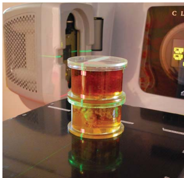
Figure 1. The two sections of the multi-modality phantom used, here aligned with the setup positioning lasers on the treatment couch prior to CBCT scan.
