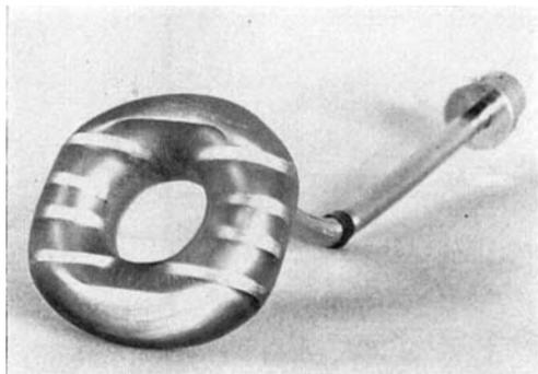
Fig. 2. The vaginal applicator of the remote afterloading unit. The gold screens and flanges are covered with araldite.
