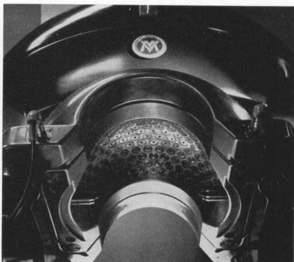
Fig. 9. The inner collimator helmet (Fig. 8), in position outside the apparatus, seen obliquely from underneath. The helmet is mounted at the operating table (Fig. 8). The horizontal spindles (coinciding with the P axis in Fig. 6) are used for fixation of the stereotaxic instrument.
