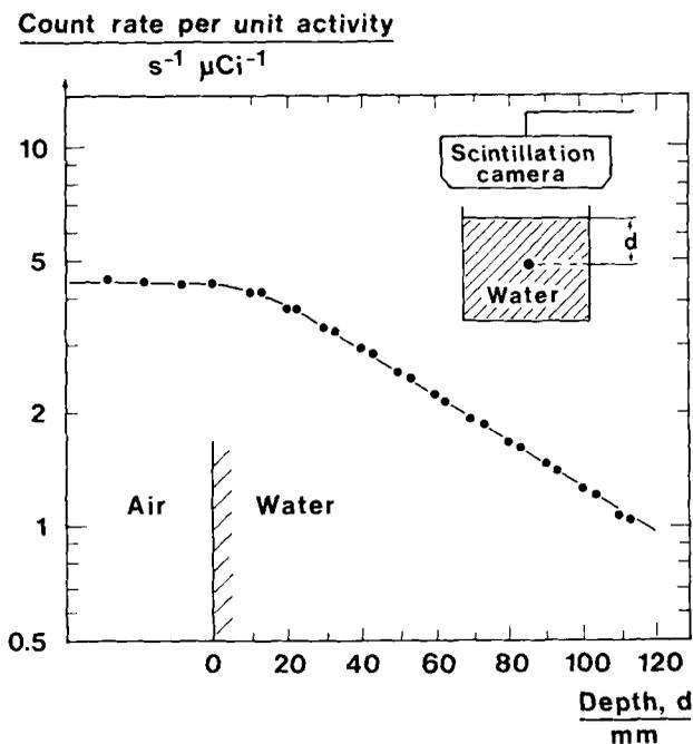
Fig. 2. Calibration factor for the lymph node phantom as a function of depth in water. The scintillation camera was equipped with a parallel 16000-hole collimator. A 35 per cent energy window was centered over the 140 keV full energy peak.
