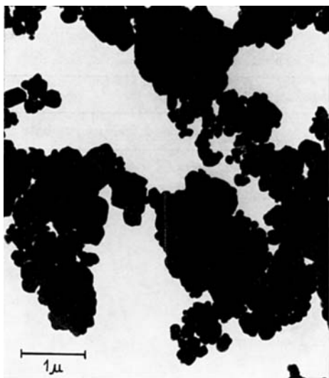
Fig. 3. Barium sulphate (preparation III) in water suspension.
