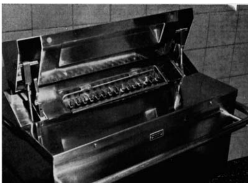
Fig. 5. The radium cart loaded with irradiators ready for use.
