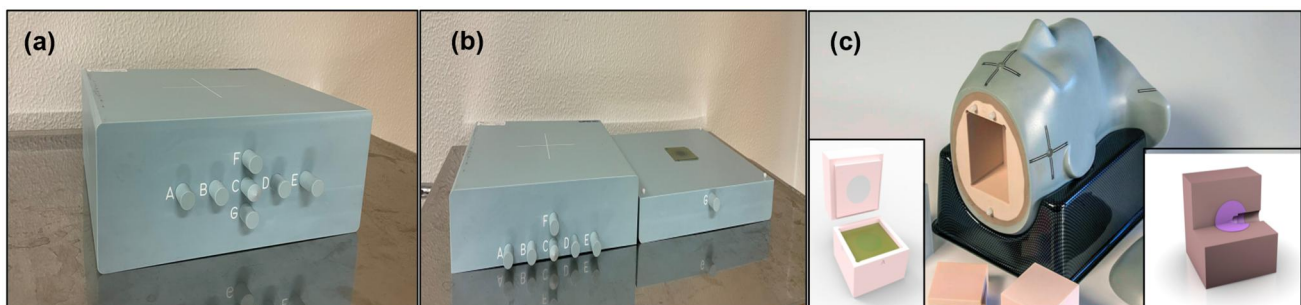
Figure 3. Phantoms used for patient QA. (a) MVP phantom assembled for irradiation. (b) Positioning of the film in the Middle of the MVP phantom. (c) The anthropomorphic STEEV phantom with the special film holder.
