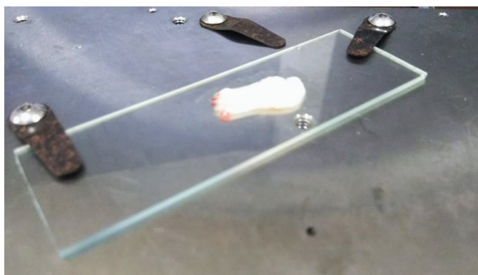
Figure 1. Sample prepared and clamped for assessment in a triboindenter.
