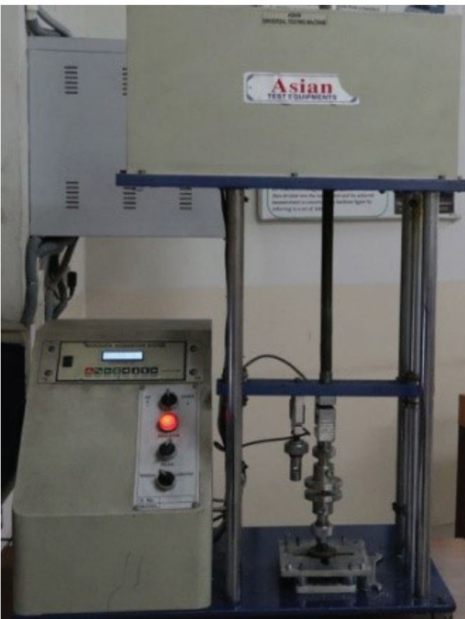
Figure 5. Universal Testing Machine setup for checking compressive strength.
