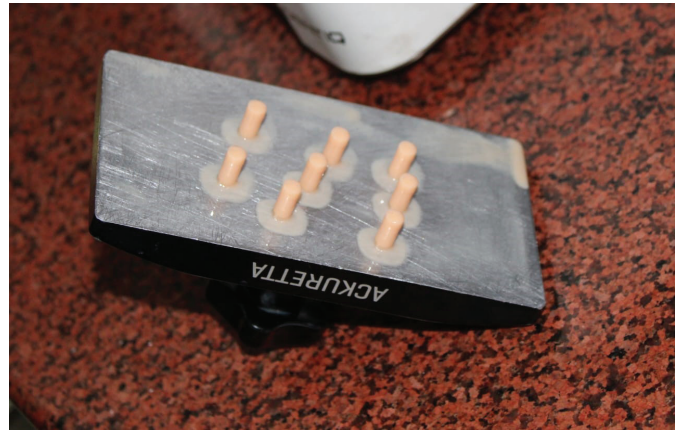
Figure 2. Cylindrical specimens fabricated for compressive strength testing.
