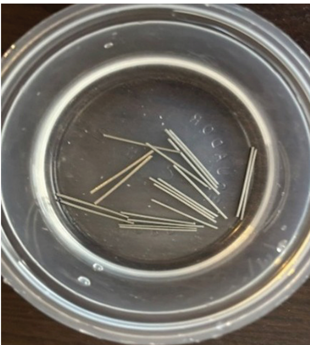
Figure 2. Immersion test in artificial saliva.
