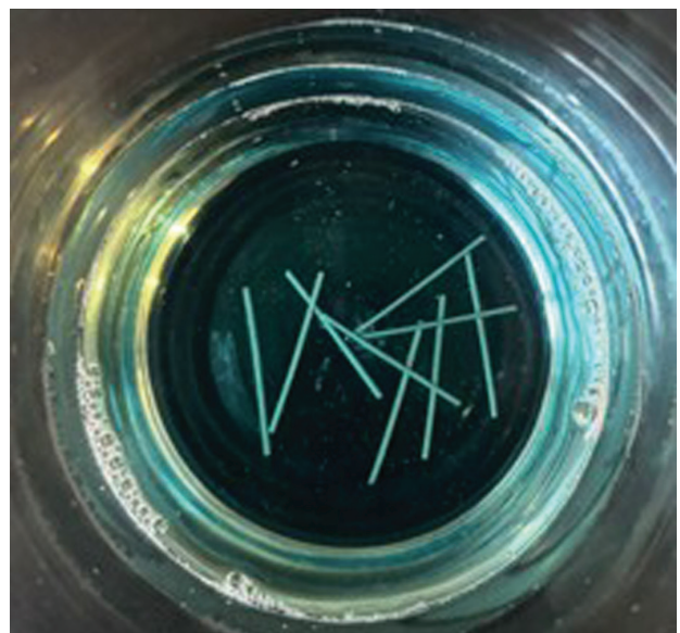
Figure 3. Immersion test in Encident Brackets mouthwash.
