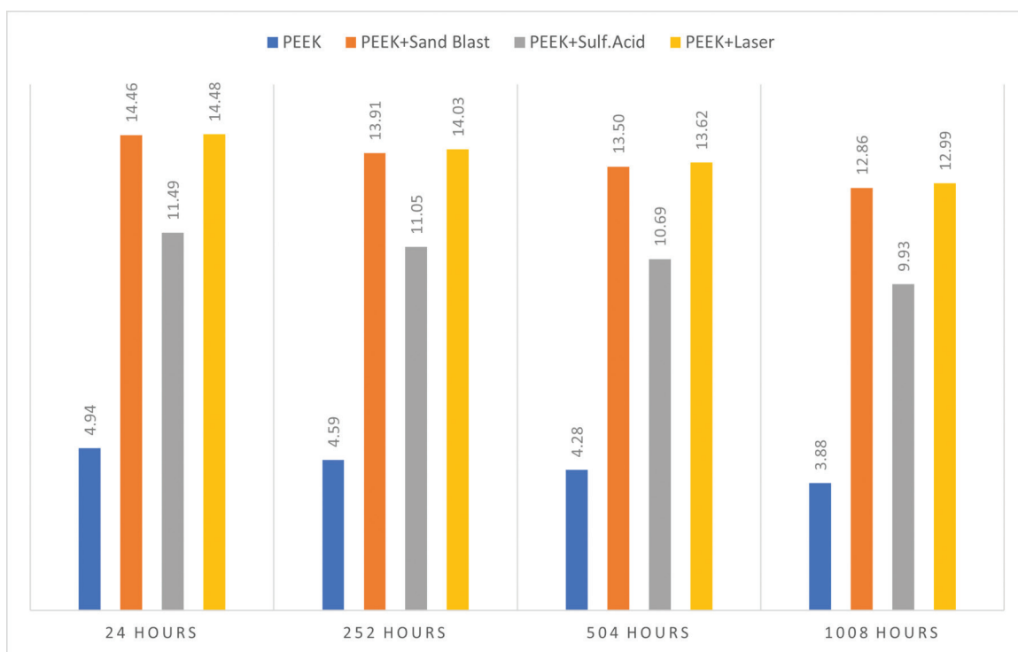
Figure 2. Inter group comparison of shear bond strength (MPa) between PEEK and maxillofacial silicone after 24 h of fabrication, 252 h to 504 h and 1,008 h of accelerated ageing.
