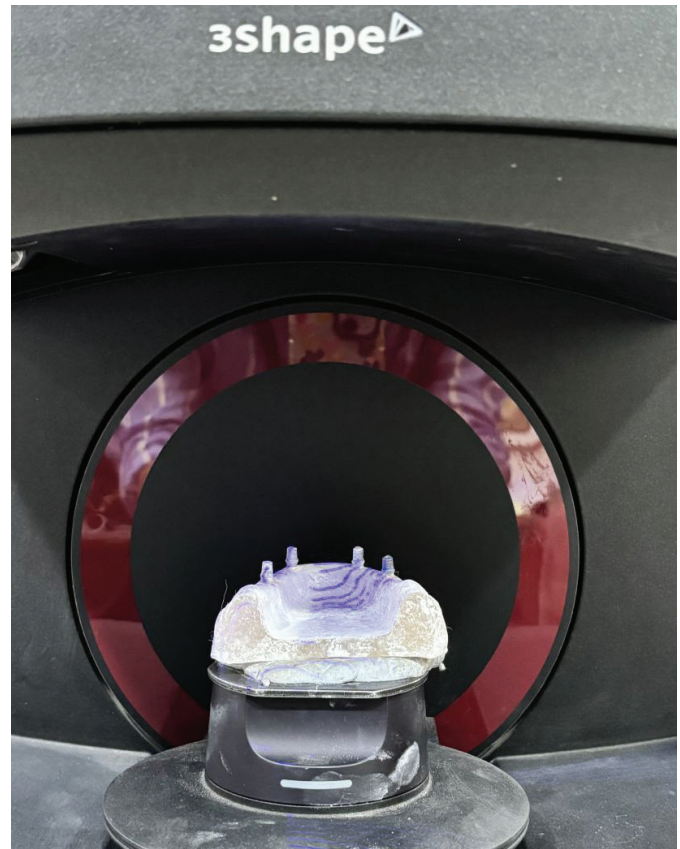
Figure 3. Scanning of implant abutments using digital lab scanner.
