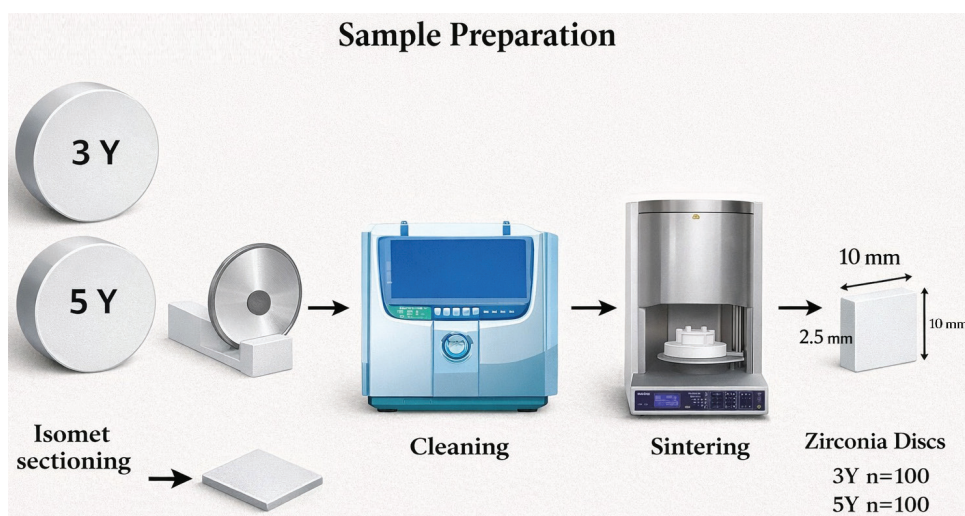
Figure 1. Diagram representing zirconia specimens' preparation.
