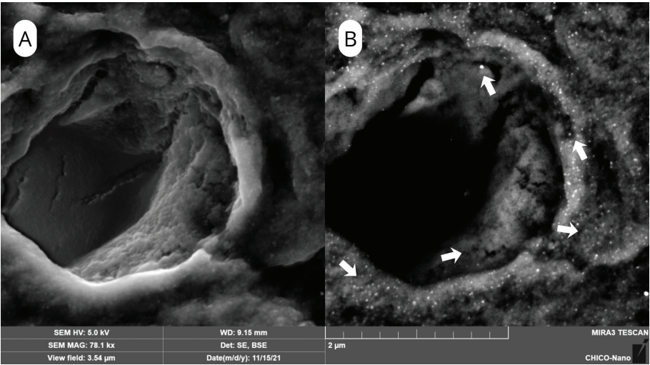
Figure 4. SEM images of dentin treated with Nano Silver Fluoride (NSF) at 1500ppm. A) SEM/SE image illustrating the dentin surface morphology; (B) SEM/BSE image showing intense and widespread silver nanoparticle deposition (arrows) across dentin surface..
