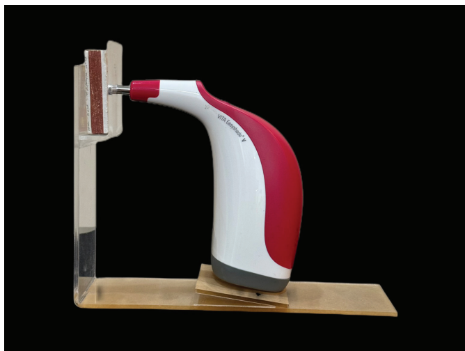
Figure 3. Device designed to ensure reproducible tooth positioning for color measurement.
