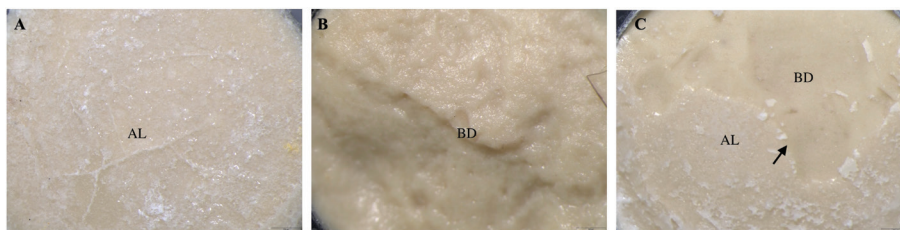
Figure 2. Representative stereomicroscopic images (×25 magnification; scale bar = 500 μm) illustrating the failure modes between Biodentine™ and restorative materials after the shear bond strength test. (BD: Biodentine™; AL: Adhesive layer). (A) Adhesive failure: Separation occurred at Biodentine™ and restorative material interface, with the adhesive layer visible at the interface. (B) Cohesive failure within Biodentine™. (C) Mixed failure: Combination of adhesive failure with adhesive layer at the interface and cohesive failure within Biodentine™. Arrow indicates the boundary between Biodentine™ and the adhesive layer.
