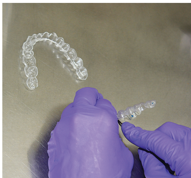
Figure 1. Samples being cut into pellets.
