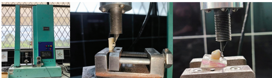
Figure 4. (A) MTS universal testing machine, model T5002; (B) Stabilization and fixation of the acrylic base in the testing machine and positioning of the stainless-steel beveled tip; (C) Direct fixation of the ceramic specimen in the testing machine and positioning of the stainless steel beveled tip.
