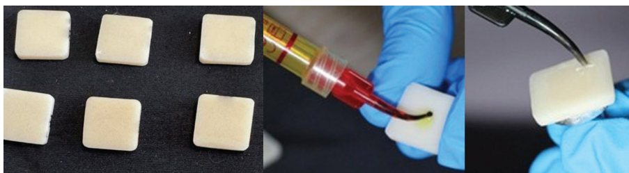
Figure 1. (A) Ceramic; (B) Surface conditioning of the ceramic with 9.6% hydrofluoric acid; (c) Application of silane on the surfaces of the ceramic.
