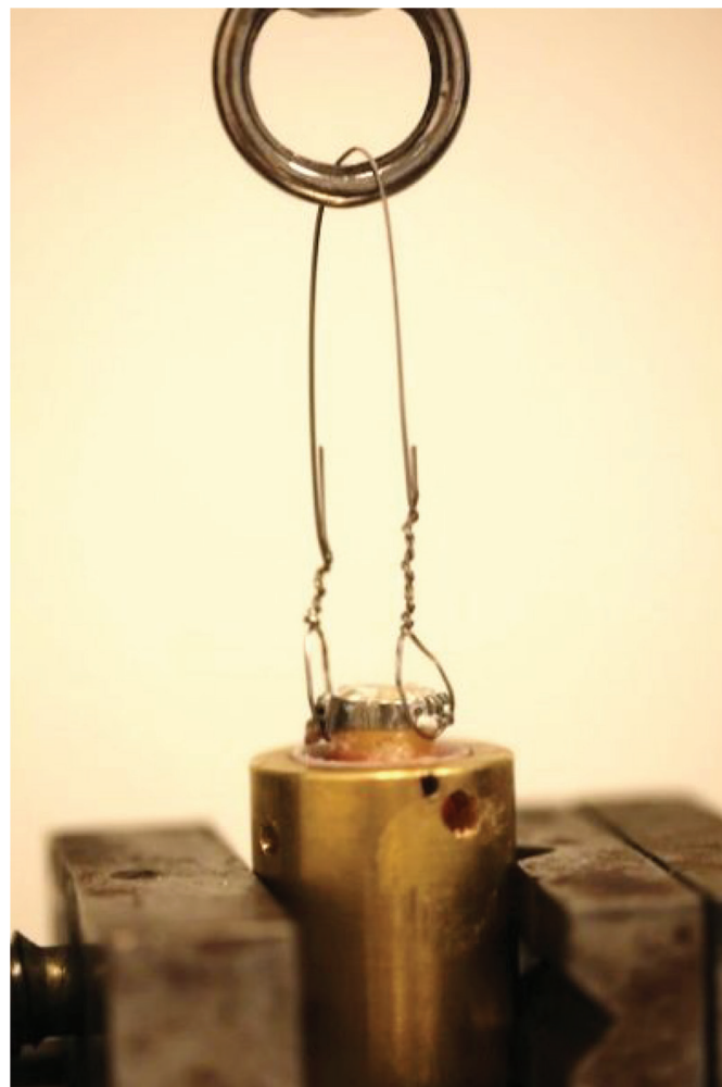
Figure 4. The loose wire through the ring makes it possible to balance the pulling force on both sides.
