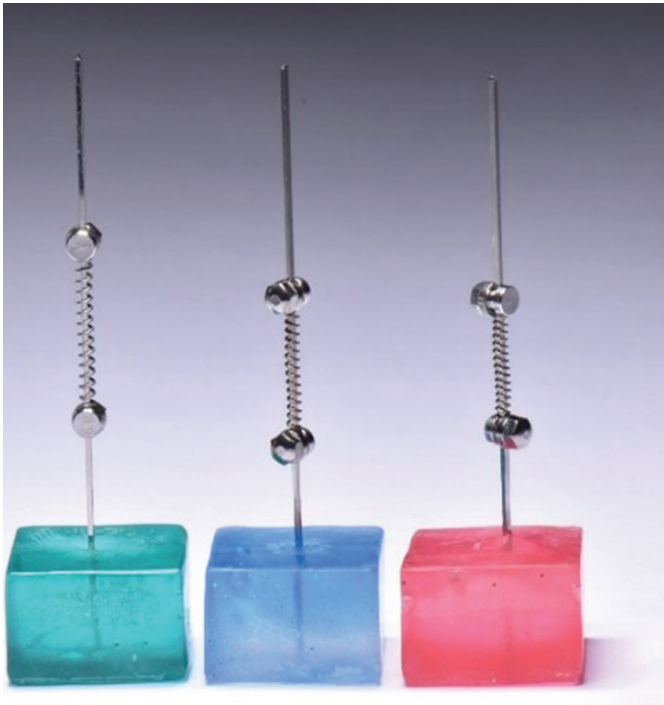
Figure 1. Acrylic cubes with springs prior to compression.
