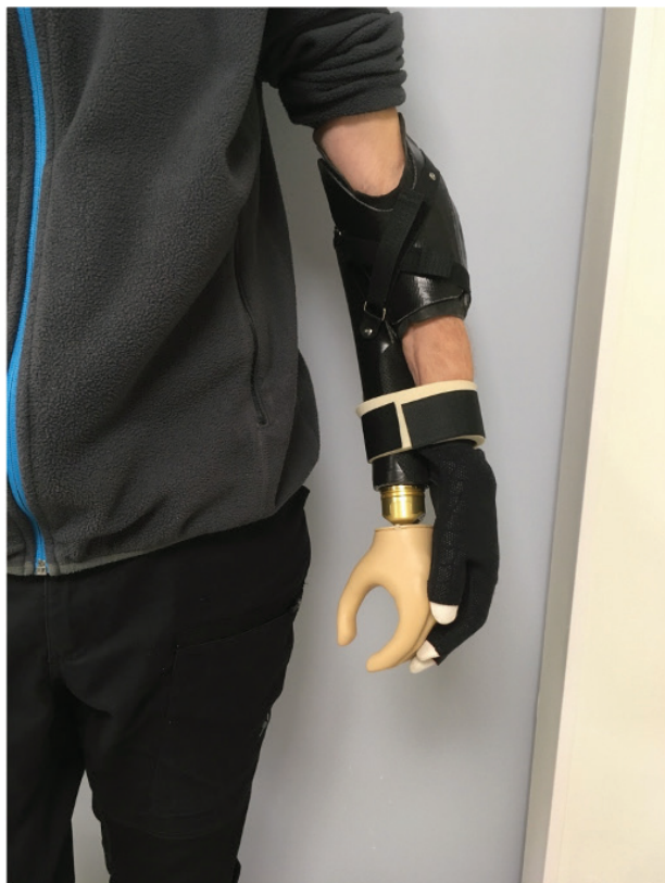
Fig. 2. The hybrid myoelectric prosthesis with a SensorSpeed hand (OttoBock) applied to the arm in the process before the amputation. This solution gave the patient the opportunity to get an idea of what he could expect from a hand prosthesis.
