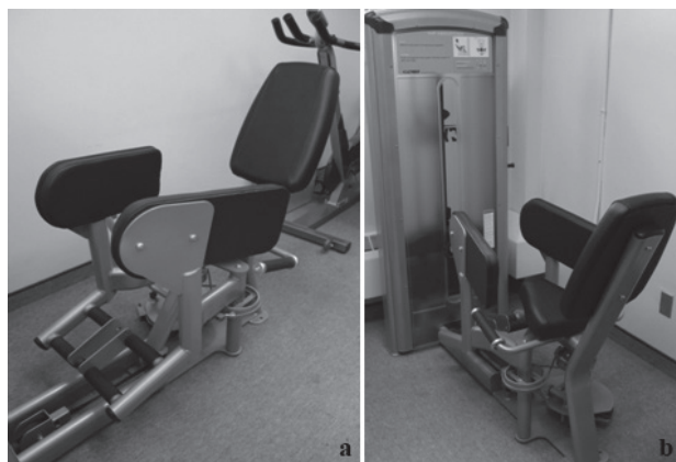
Fig. 2. Modified hip abductor machine (Cybex International, Inc.), indicating elongated hip abductor pads. Figs 2a and 2b show the anterior and posterior oblique views, respectively, of the modified hip abductor.
