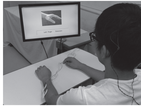
Fig. 1. Training with brain computer interface–neuromuscular electrical stimulation. The subject attempted to extend his fingers according to the instructions presented on the monitor. Electrical stimulation was triggered if the amplitude of the motor-related cortical potential reached a pre-determined threshold.
