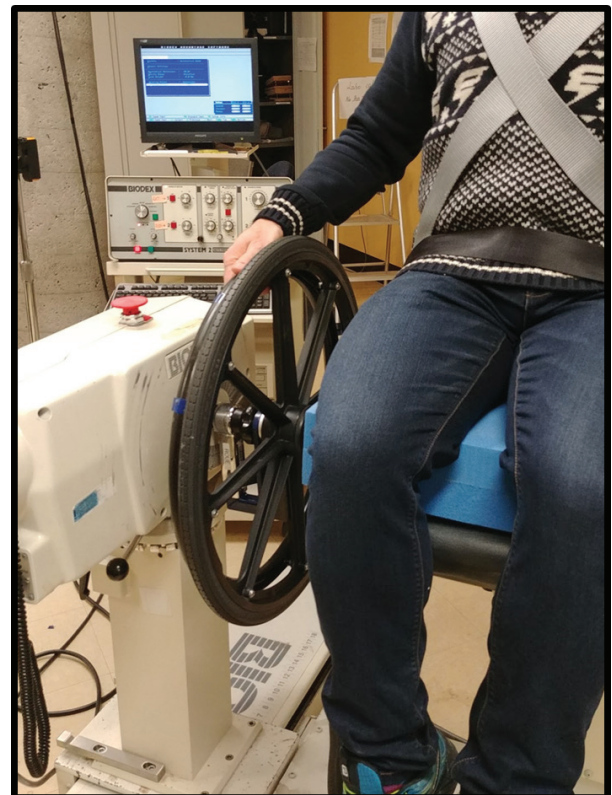
Fig. 2. Wheelchair wheel adapted to become mountable onto the shaft of an isokinetic dynamometer system.
