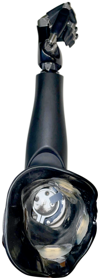
Fig. 5. Osseointegrated socket prosthesis with four active electrodes (and one inactive electrode) in patient 2.
