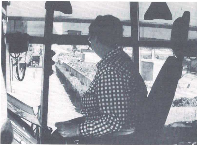
Fig. 1. The crane operators all had a forward tilted sitting position causing high static loads upon the neck and shoulder-stabilizing muscles.
