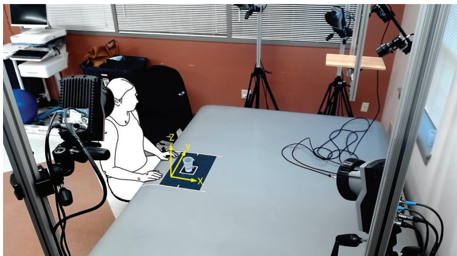
Fig. 2. Motion capture setup. To measure kinematics of the drinking task activity, 5 optoelectronic cameras measured motion of skin-adhered markers relative to the depicted origin and cardinal plane.
